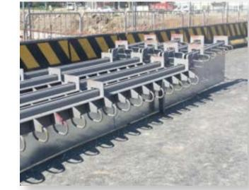
Arfen single-span steel expansion joints are used in transverse direction at the bridges, with a total movement capacity of 80 mm or 100 mm, the bearing assembly is connected to the structure by means of the ropes and the rubber strip sealing element for water tightness is used. The steel profiles in this system can consist of extrusion profiles.
