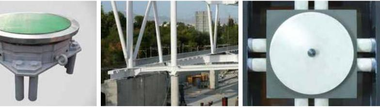
This type isolator works with the energy damping principle by friction. If the seismic forces acting on such isolators exceed the static frictional force limit, the steel sphere in the isolator begins to slip on the concave bottom plate. Then the isolator allows the structure to oscillate like a pendulum.
